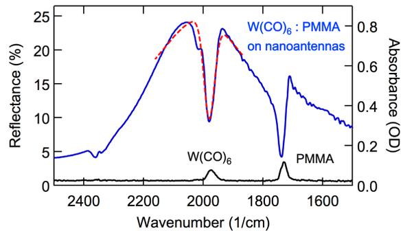
Figure 2. The reflectance spectrum for nanoantenna arrays covered with the sample film (blue line) and the absorbance spectrum for a  $\text{W}(\text{CO})_6$ -dispersed 200-nm thick PMMA film (black line).
