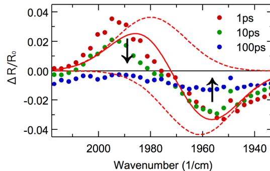
Figure 3. Transient reflectance-change spectra for  $T_{1u}$  C=O stretching mode of  $\text{W}(\text{CO})_6$  with nanoantenna arrays. The red solid line represents a fitting curve composed of two Gaussian bands (red dashed line).
